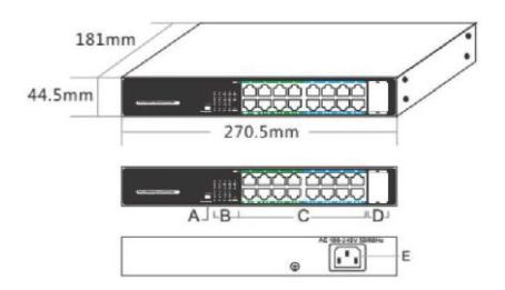
A.Multi-functional switch B.Working LED indicator
