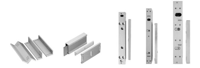
Discovery's DEB-02 high quality magnetic locks are ideal for secure applications where access is restricted, such as office buildings, hospitals, and airports. They have a holding force of 300/600/1200 pounds, respectively, and are easy to install. The attractively designed Maglocks are surface mounted, operate on dual voltage, 12 VDC or 24 VDC, and have low current consumption. These Maglocks are compatible with EN and UL standards.
